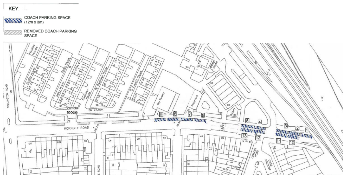
Proposed coach parking layout for Hornsey Road – showing 13 spaces with double stacking.
